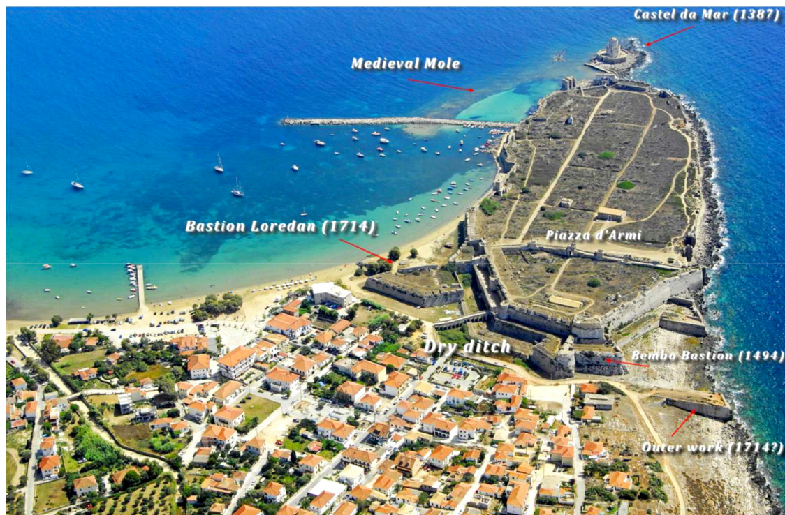
6. Aerial photography of Modon from the north and labeled, land front, August 2007.
