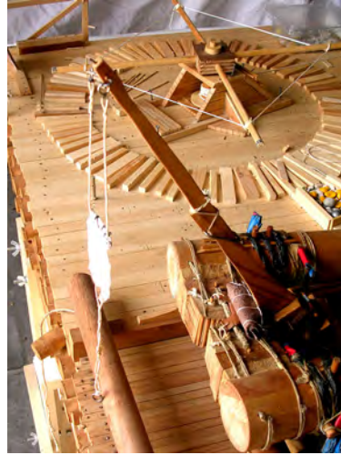
Fig.26: Another scale-model of Version- 2B at rest, the arm lies loosely on the leather cushion.
