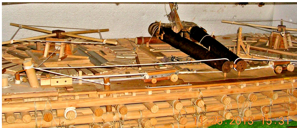
Fig. 29: A model of Version-2B, with the bogie-tackles upon the slide-table of the fulcimentum.
