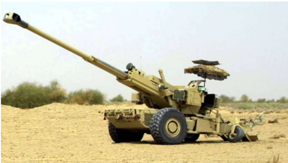
Fig. 6. 155mm Bofors Fälthaubits (Swedish for ‘Field Howitzer’) FH77/B02. After the weapons contract scandal, the original plan for acquisition of more than 1,000 examples was scrapped, instead, the Indian Army acquired only 410. In service with about 20 artillery regiments by 1999, it proved highly successful during the Kargil War partly because of its range of 38 kilometres (when using base bleed-rounds generally).
