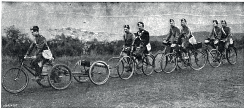
A motor cycle, with Maxim gun attached. Cyclists in rear carrying ammunition.
