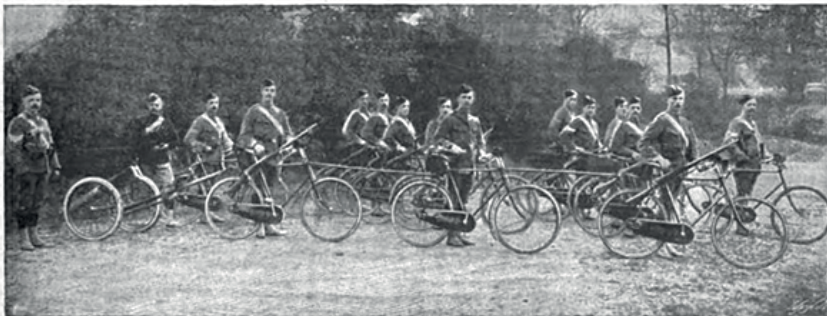
Bringing a Maxim into action, drawn by three cyclists whose machines are connected by a light rod with the gun-carriage.
