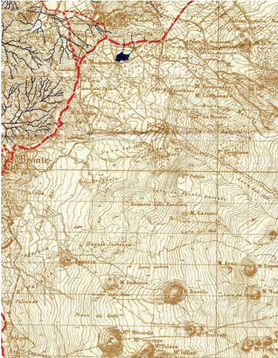
Fig.8 Detail of the 1:50,000 Bronte sheet (261-II) G.S.G.S. 4229, M.D.R. 578/8152 Second Edition (Coloured) dated May 1943. This map is a brown “griblet” with the water features over-printed in blue and roads in red. The reprographic material for the brown plated was supplied by the War Office, but the red and blue plates were produced in Egypt. (Author’s collection)
