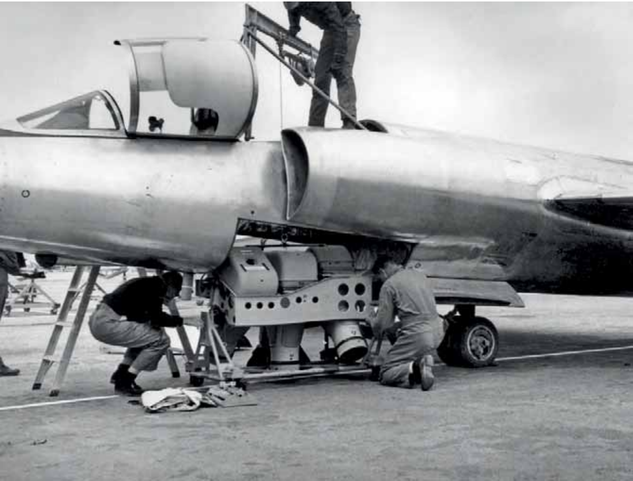
Fig. 16 Technicians load a Hycon 73B camera into a U-2's equipment bay. (U.S. Air Force photo).
