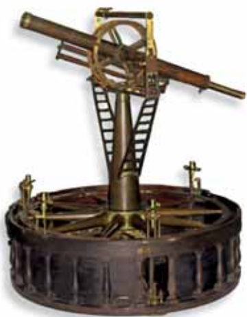
3-foot ramsden theodolite from 1791 used during the principal Triangulation of Great Britain. Noe in the Science Museum, London. Photo by User.geni, December 2008. CC-BY-SA GDFL
