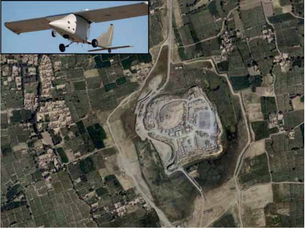
Fig. 21 The US Buckeye Unmanned Air Vehicle is able to take digital imagery on the ground at 10 cm resolution. In the larger image, a view of the Indo-Parthian settlement of Spirwan Ghar in Qandahar Province, Afghanistan, which was obliterated by a military infrastructure. (From Elena LEONI, « Geospatial Accuracy Matters! A preliminary study about the impact on CP in Afghanistan », paper presented at Penn Cultural Heritage Conference, 2017)
