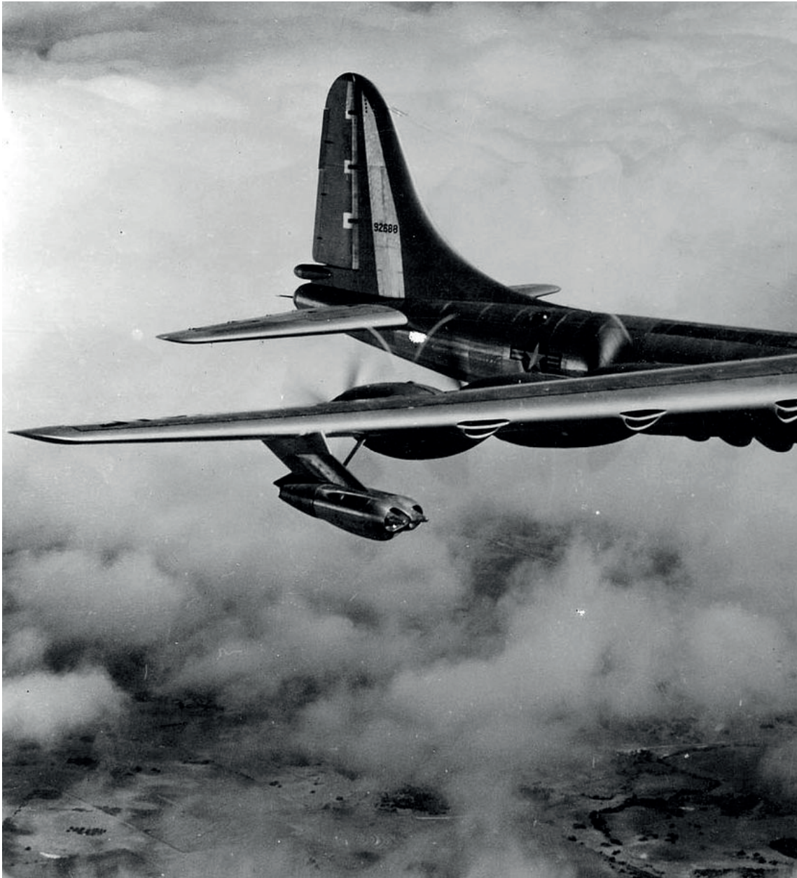
Fig. 15 The first strategic reconnaissance aircraft was the RB-36D specialized photo-reconnaissance version of the B-36D. In the smaller image, a K-42 Camera, nicknamed “Pie Face” or the “Boston Camera”. (Image modified by authors).
