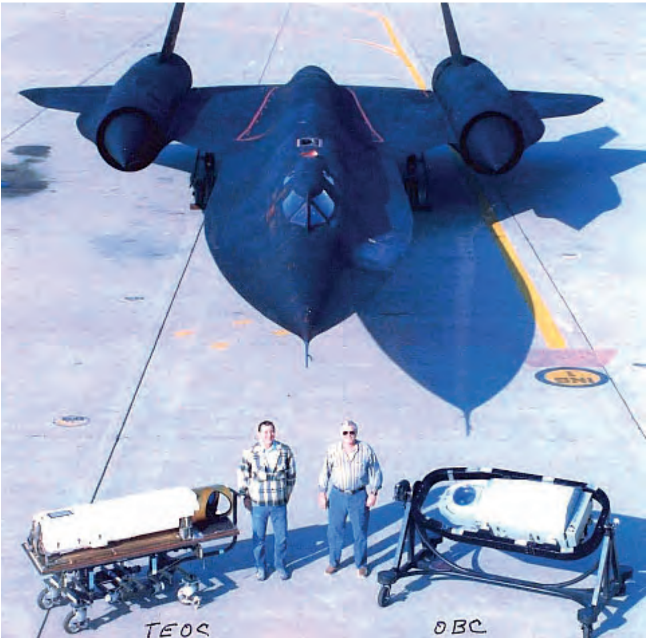
Fig. 17 On the foreground of Lockheed SR-71 “Blackbird”, there are its main photographic sensors: the Technical Objective Camera TEOC and the Optical Bar Camera (OBC). (Photo Courtesy Dave Nolte, Boeing).
