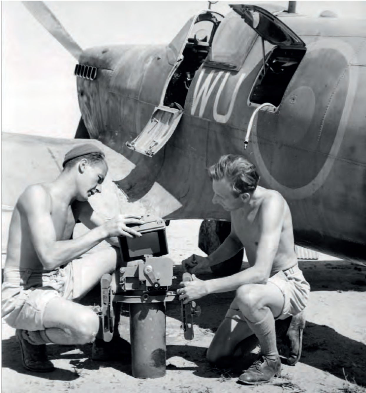
Fig. 9 This image shows a RAF photographer fitting two F24 cameras into a Mk Ic Photo-Reconnaissance Spitfire in 1939-1940. ( https://www.militaryimages.net/media/spitfire-cameras.7515/ )
