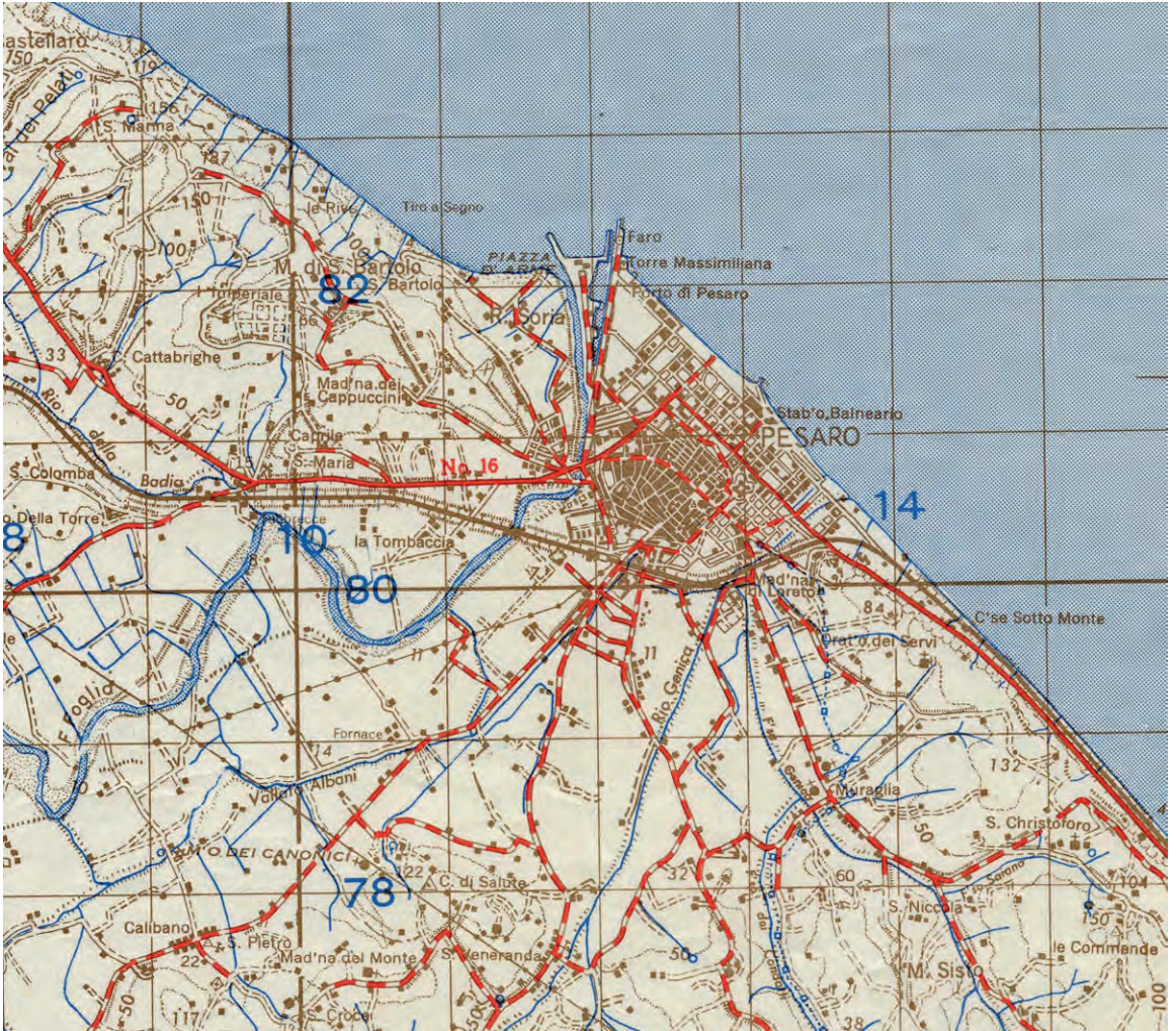
Fig.10 Detail of the 1:50,000 Pesaro sheet (109-I), G.S.G.S. 4229, A.F. 14598, Fourth Edition printed and revised by 13 Corps. Field Survey Company Royal Engineers in July 1944, but using reprographic material produced in 1943 by A.M.S. The brown and blue plates shows the improved quality of the American drawn maps despite being printed in “griblet” form. (Author’s collection)
